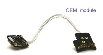
The **CLC** lens controller for Canon EF and EF-S mount type lenses provides for aperture, focus and stabilization control. It can operate as a stand alone device, powered though serial control or as an embedded device using RS232, UART, or as an I2C controlled component. A USB to UART cable allows for USB operation.
